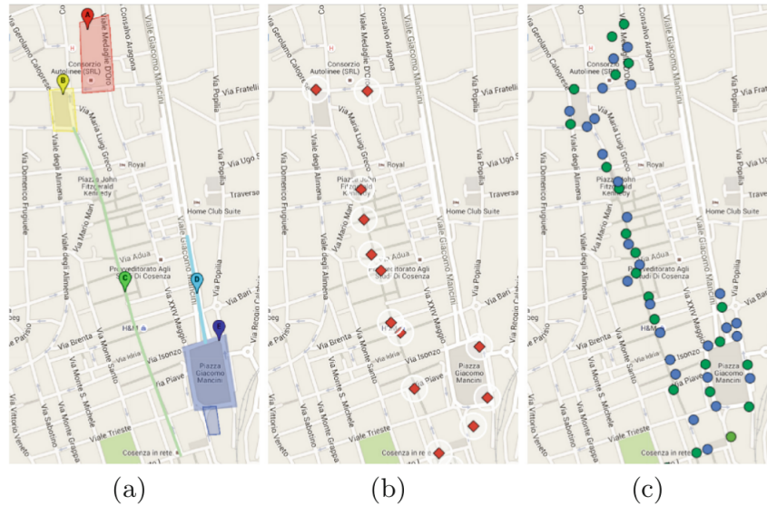
Smart Street Cosenza. (a) Target areas; (b) Computational Nodes; (c) Sensors nodes. Green locations host one type A node and one type B node, blue locations hosts only a type A node.
