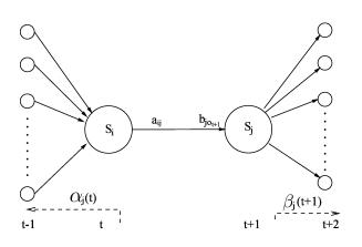
Given an observation O, the model  $\mu$  Probability  $\varphi_t(i,j)$  of moving from state  $s_i$  at time t to state  $s_i$  at time t + 1 given observation O.
