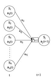
Closeup of the computation of forward probabilities at one node. The forward probability  $\alpha_j(t+1)$  is calculated by summing the product of the probabilities on each incoming arc with the forward probability of the originating node.
