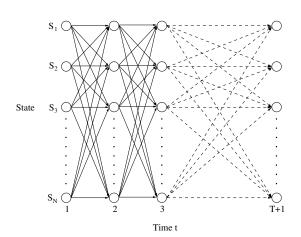
Fully connected HMM where one can move from any state to any other at each step. A node  $\{s_i, t\}$  of the trellis stores information about state sequences which include  $X_t = i$ .
